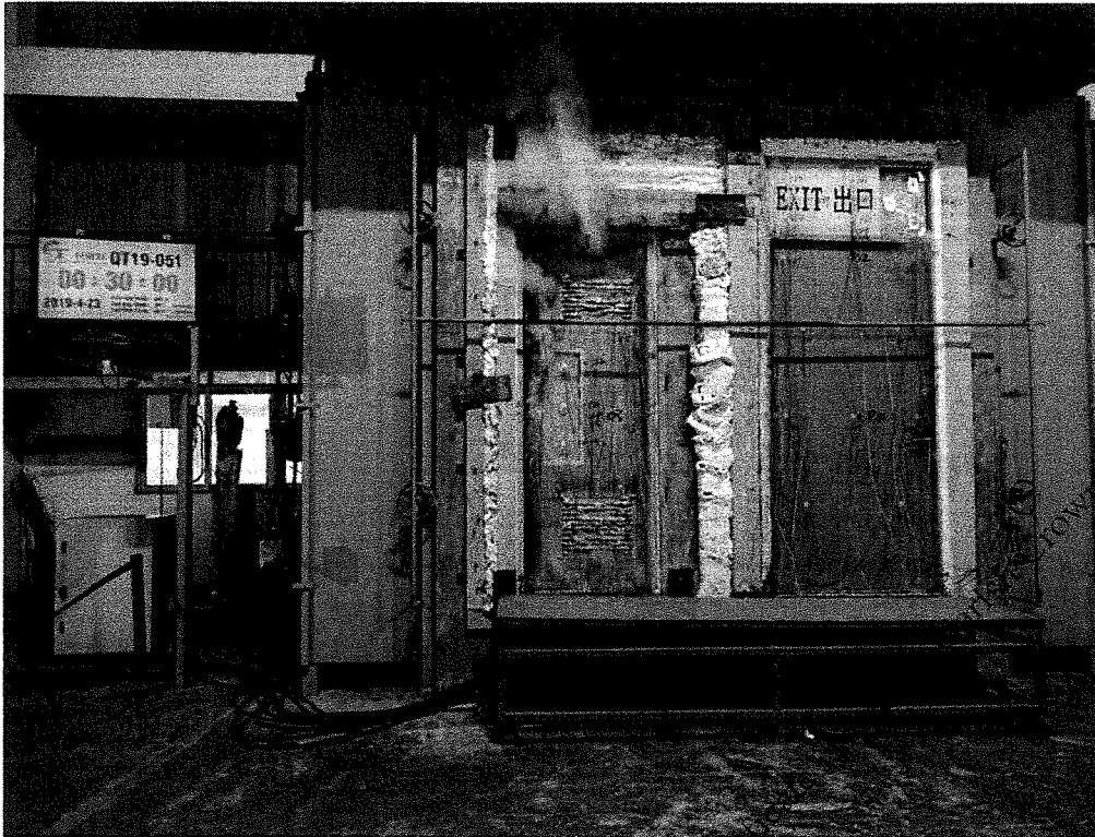
Photo 3. Unexposed surface of the specimens at 30 minutes of test.
