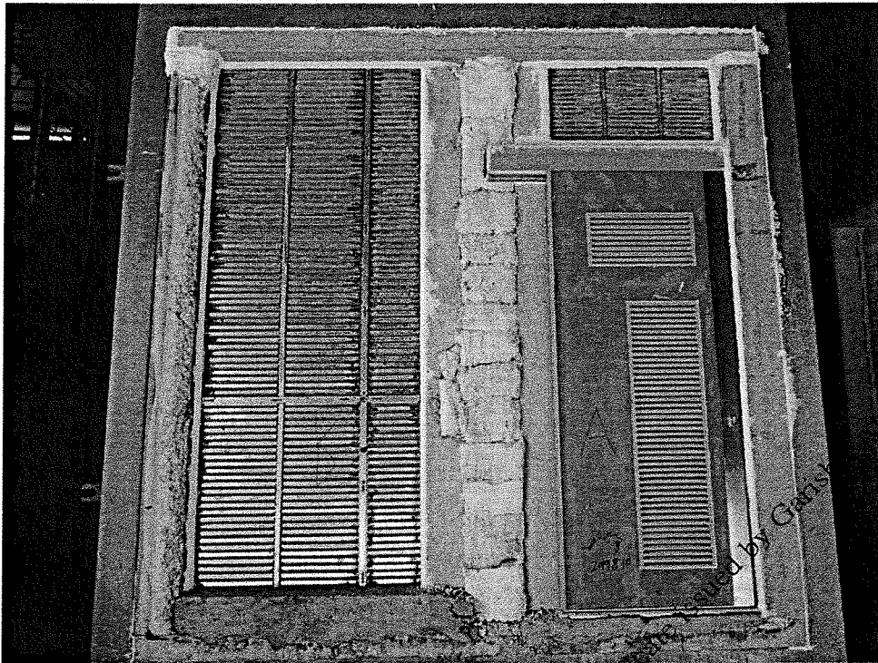
Photo 1. Exposed surface of the specimens before test. (Left: Louver B; Right: Door A and Louver C)
