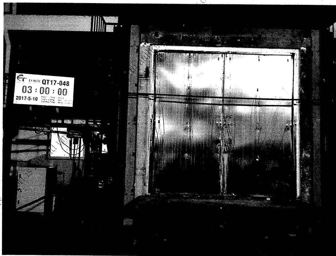
Photo 8. Unexposed surface of the specimen at 180 minutes of test.
